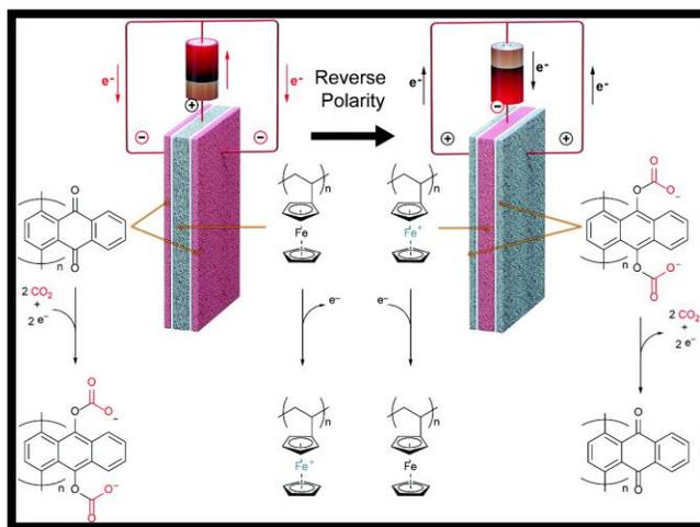
**Figure 10-** Diagram of Faradaic electro-swing reactive adsorption electrochemical cell and the chemical reactions it performs from the original article [10].
