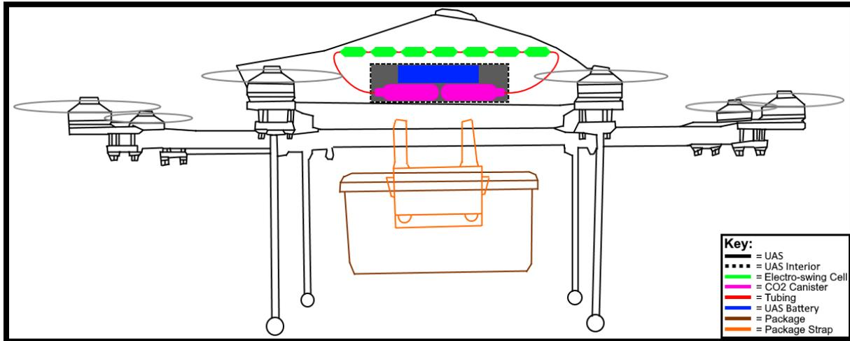
**Figure 14-** Schematic of an Amazon Prime Air UAS modified with the inclusion of Faradaic Electro-Swing Reactive Adsorption Electrochemical Cells and CO<sub>2</sub> tanks; this is a potential design for a next-generation UAS [33]; air currents created by the blades of the UAS or an air pump are two possible methods for funneling in CO<sub>2</sub>.
