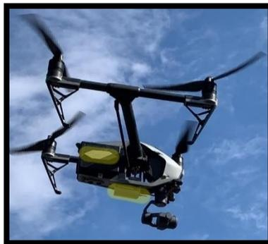
**Figure 16-** Test flight of the modeled Faradaic Electro-Swing Reactive Adsorption Electrochemical Cells on a DJI® Inspire 2.
