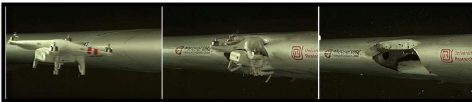
**Figure 8-** Demonstration of the impact of a high-speed collision of a UAS and an airplane wing [19].
