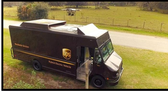
**Figure 12-** Shown above is another commercial use of UAS, which is UPS using a UAS to complete a delivery of a package. The UAS serves as a supplement, rather than a replacement, to a standard delivery truck [32].
