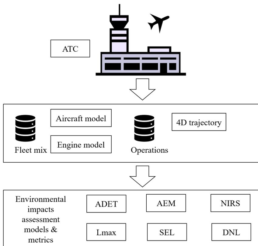
Figure 1. Noise prediction process for towered airports (FAA, 2017a)
