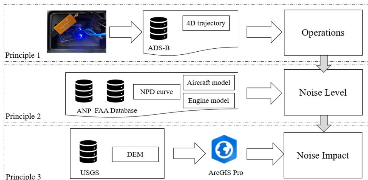
Figure 2. Diagram of the proposed noise prediction approach layout
