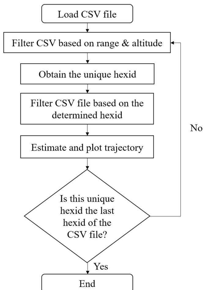
Figure 5. Flowchart of estimation of aircraft operations using ADS-B
