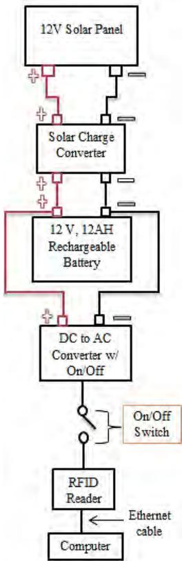
Figure 10: Block diagram of Drone Detection System electronics.
