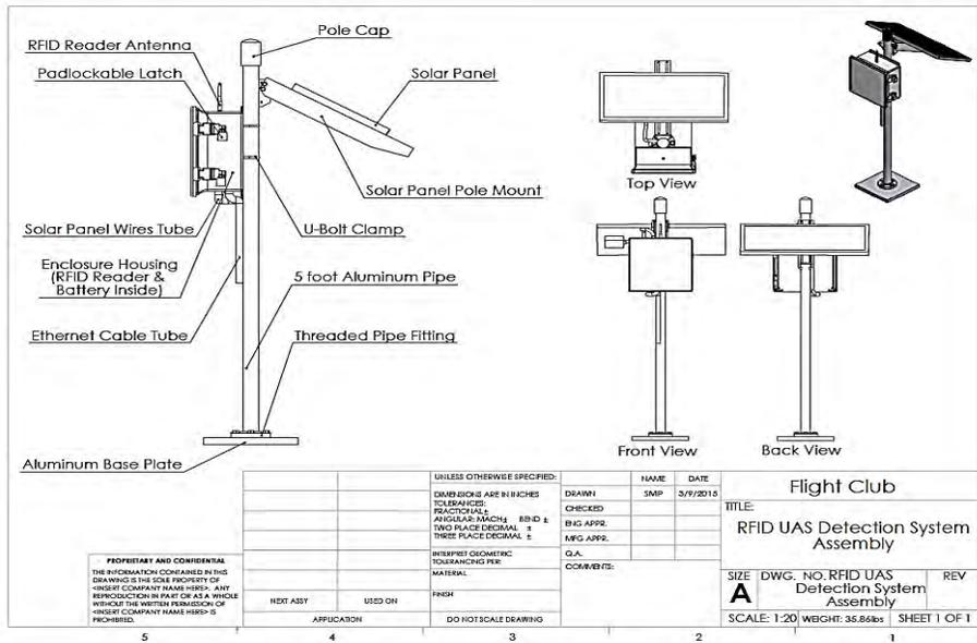
Figure 11: SolidWorks drawing of Drone Detection and Tracking System.
