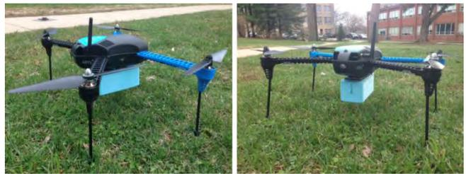
Figure 12: Drone Operator Notification System transmitter housing attached to the drone.
