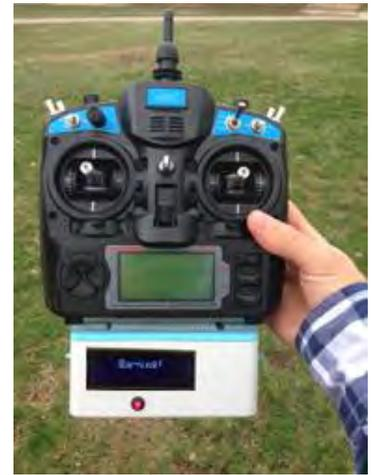
Figure 3: Drone Operator Notification System providing warning to drone operator within safety zone.
