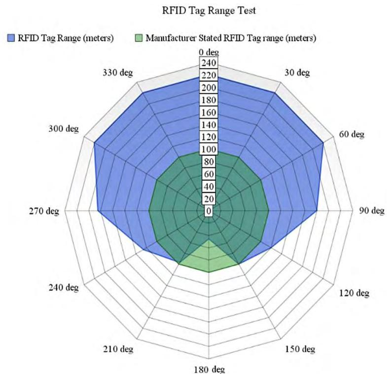
Figure 2: RFID Reader/Tag Read Range Test results.
