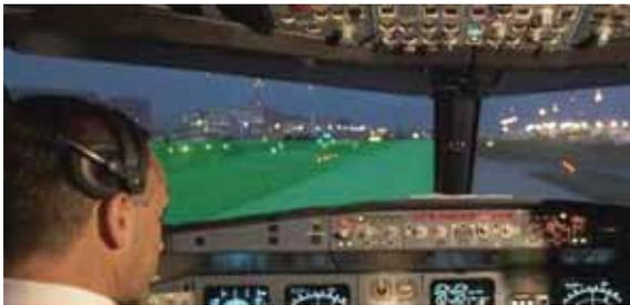
**Figure 14** - The area of vision most important to a pilot during a laser attack is highlighted in green [35]
