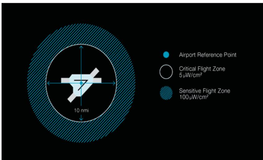
**Figure 2** - The "critical flight zone" around an airport [11]
