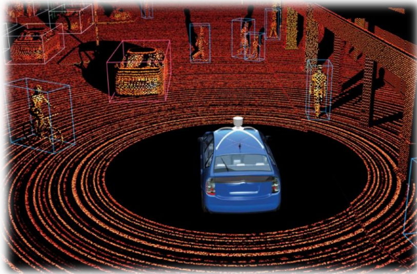
Figure 2: LIDAR scanning representation
