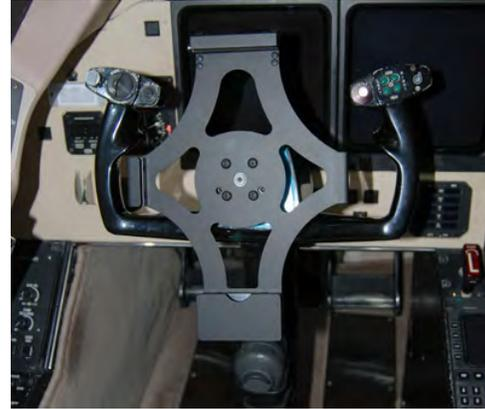
**Figure 6-2. Yoke Mount Fully Installed**
