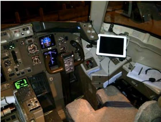
**Figure 6-3. Mounting Solution for Commercial Aircraft**
