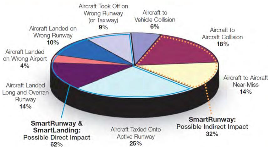
**Figure 1-6. Common Causes of Runway Incursions and Excursions (Honeywell, 2010)**
