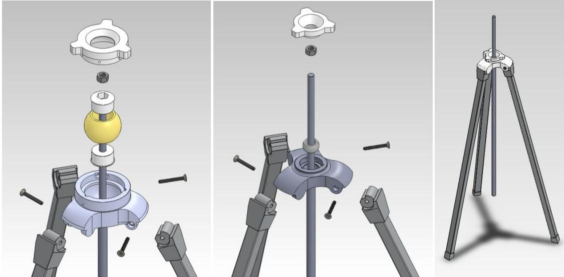
Figure 4: CAD Images of the Self-Leveling Base
