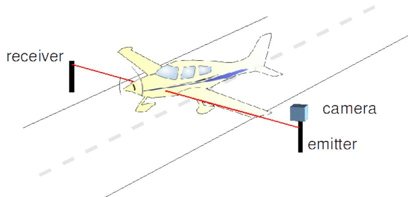
**Figure 2: Photoelectric Beam Sensor System**
