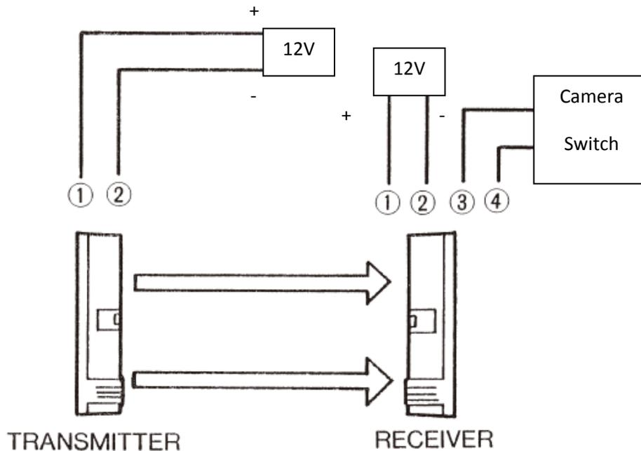
Figure 13: Sensor Wiring Diagram
