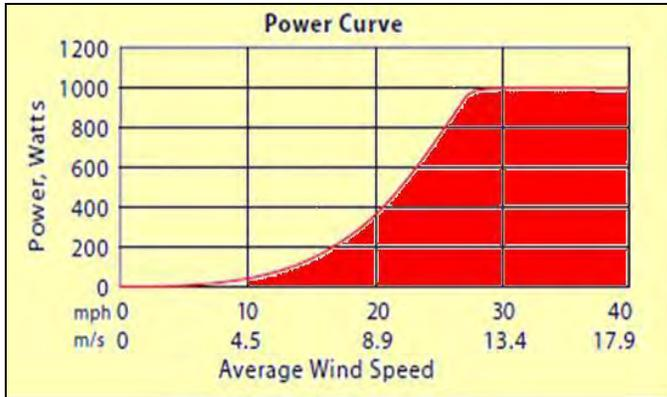
**Figure 2-2 Wind Speed Power Curve**
