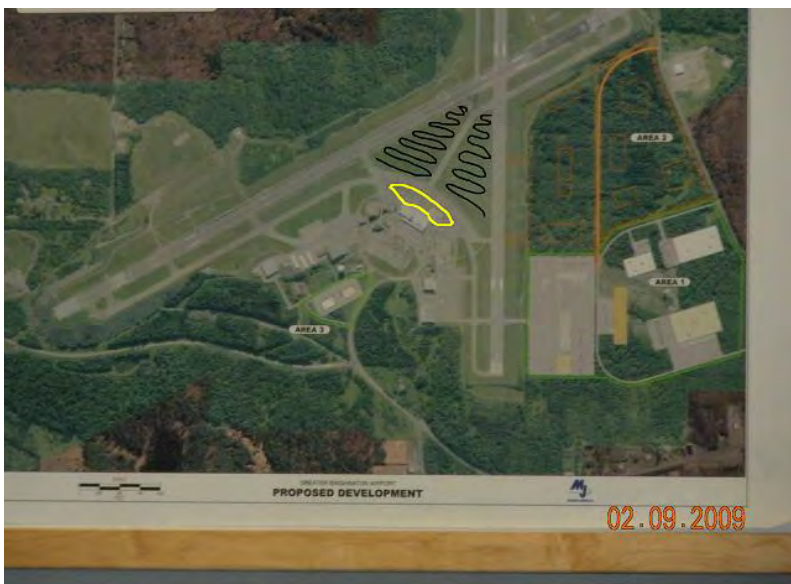
Figure 6 - Pavement to be heated and location of geothermal trenching at BGM
