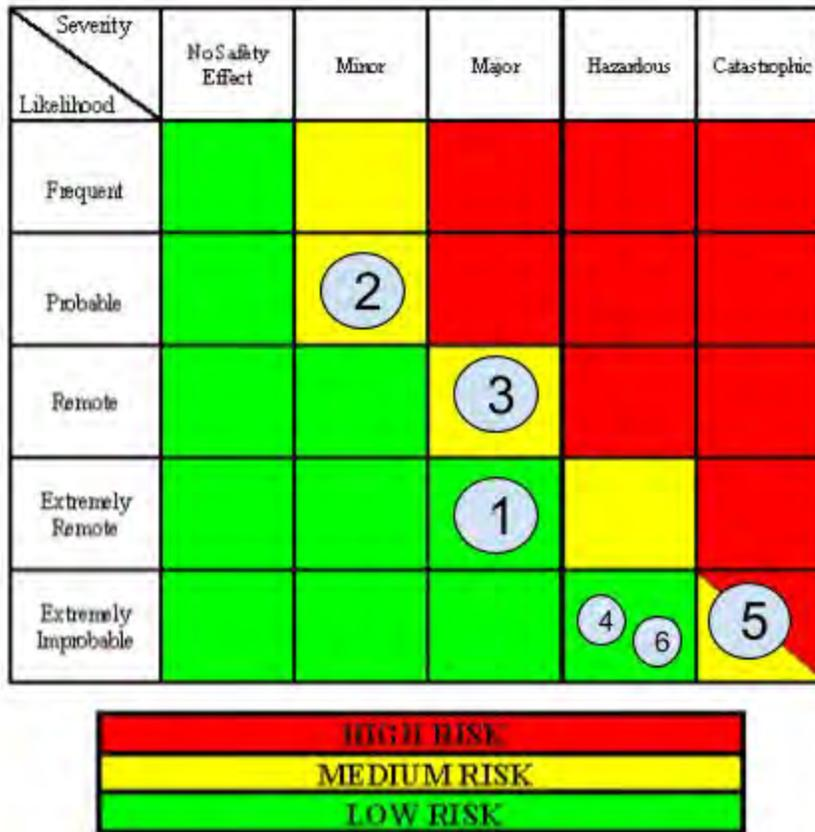
In Figure 8.4 above, Team Pro-motion has determined that the risks and hazards associated with the Transtag are medium to low, the most catastrophic risk would be associated with the ground crew being badly oriented towards the solution.
