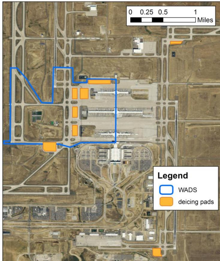
**Figure 1.2.** Map of the West Airfield Diversion System and deicing pads at DIA.
