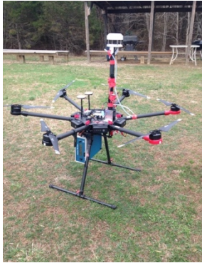
Fig. 1. Modified hex-rotor UAV with mounted O 3 analyzer and anemometer.
