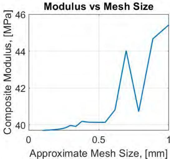
Figure 4. Effective modulus as mesh size is decreased. Note that at mesh size of approximately 0.2mm the modulus has converged.
