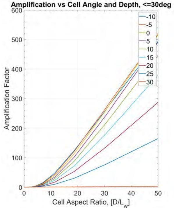
Figure 9. Effect of cell depth on amplification factor.
