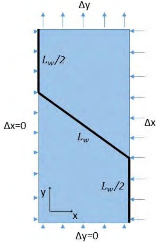
Figure 3. Cross section of unit cell rigid model and boundary conditions.
