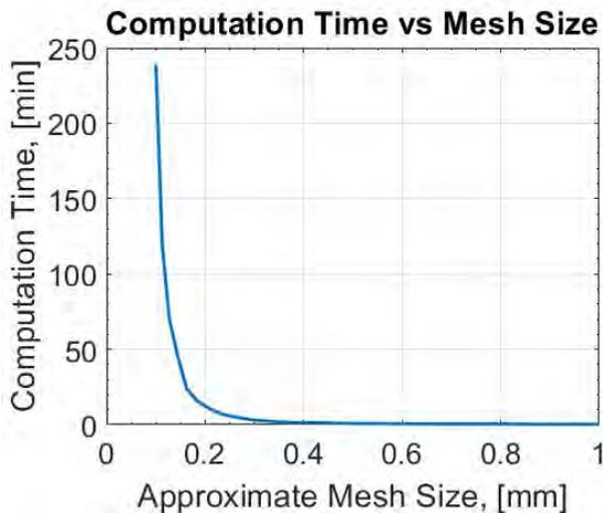
Figure 5. Computation time as mesh size is decreased. Note that after a mesh size of 0.2mm the computation time diverges and becomes impractical to solve.
