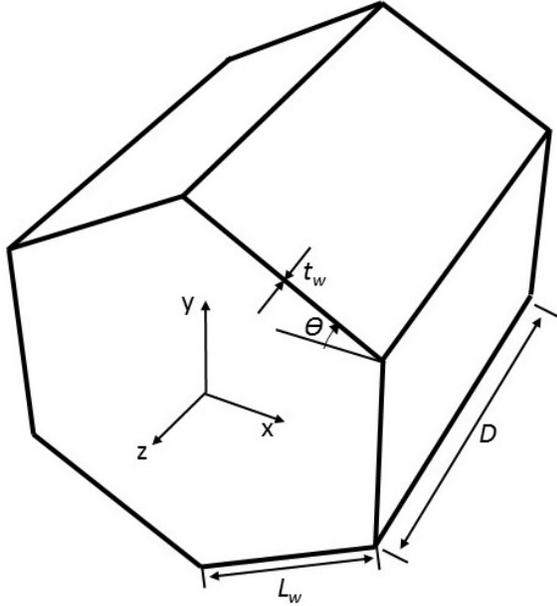
Figure 2. Definition of unit cell geometry.
