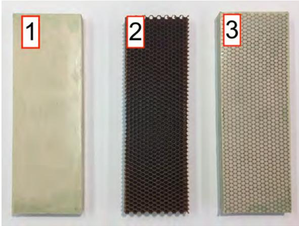
**Figure 1. HPC diagram. Polymer in (1), unfilled aramid honeycomb in (2), and polymer-filled honeycomb composite in (3).**
