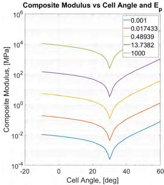
Figure 6. Composite modulus vs cell angle for constant values of polymer stiffness.
