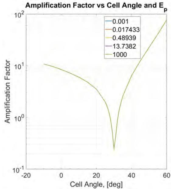
Figure 7. Amplification factor for varying cell angle at constant polymer stiffness.
