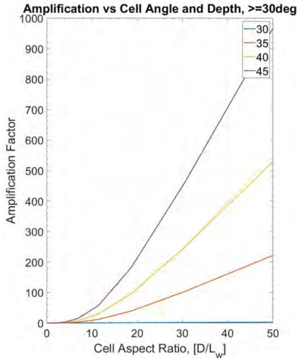
Figure 10. Effect of cell depth on amplification factor for cell angles above 30°.
