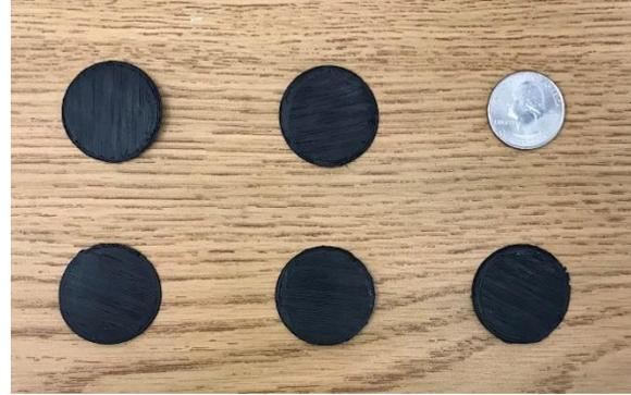
Figure 4. Nylon-LSM printed samples.
