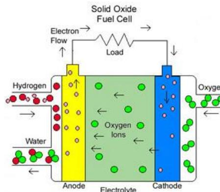
Figure 1. Electrochemical process of the solid oxide fuel cell (SOFC)<sup>1</sup>.
