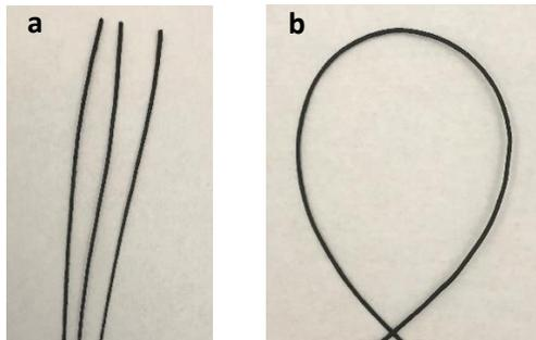
Figure 3. a. Nylon-LSM filament; b. flexibility of filament.
