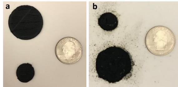
Figure 5. a. Before sintering; b. after sintering.
