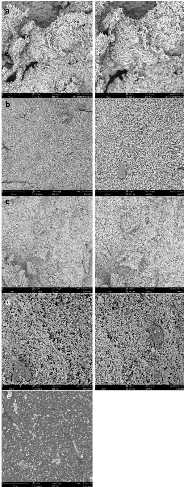
Figure 6. Sintering procedure from Table 1: a. 1, b. 2, c. 3, d. 4; e. green state sample.
