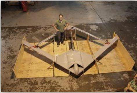
**Figure 12 - Rigid RPV in the Assembly Jig**
