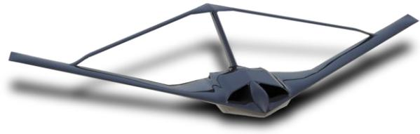
**Figure 1. Joined wing SensorCraft Concept**
