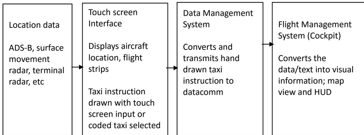
Figure 1 Design overview of Touchscreen Airtraffic Management System (TAMS)
