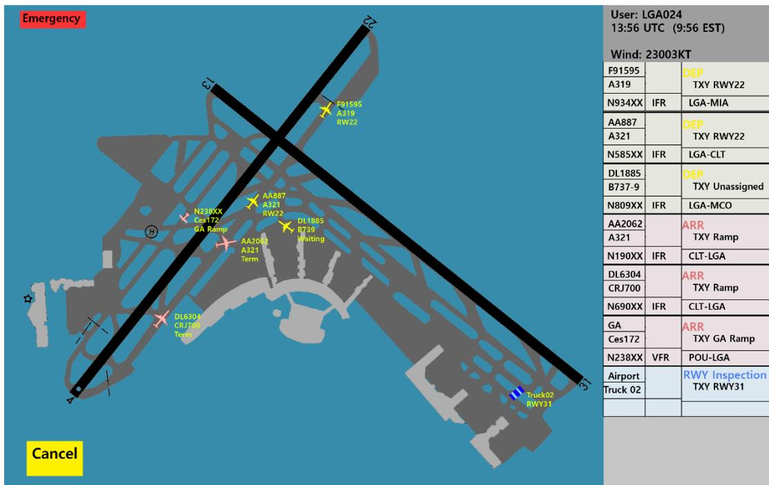
Figure 2. Touchscreen Airtraffic Management System (TAMS) user interface
