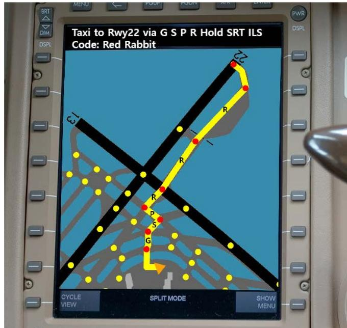
Figure 5. TAMS taxi instruction display on an electronic flight bag of B777-200\*
