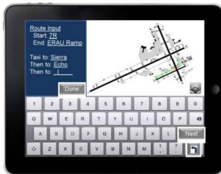
**Figure 5:** An iTaxi mock-up of route input and guidance.
