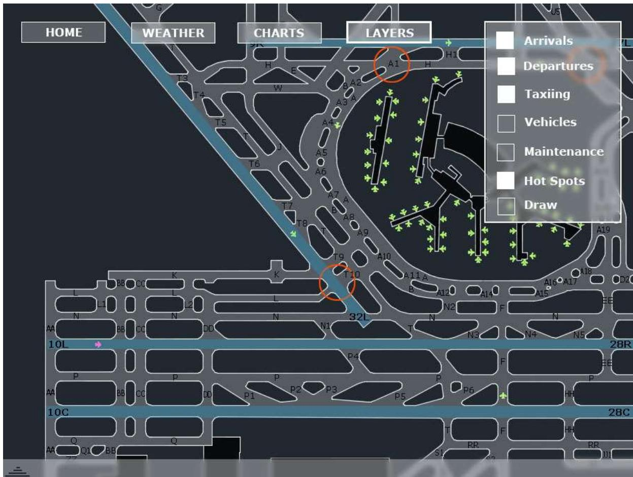
**Figure 7:** Home screen with layers tab activated.
