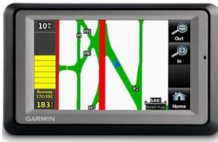
**Figure 1:** Garmin SafeNav displaying runways, taxiways, and current location.
