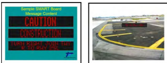
Figure 14 From the ALPA report, shows an example of what changeable LED signage could look like on the airfield.
