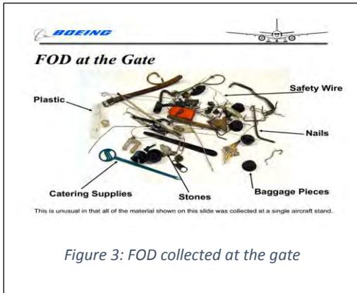
one side of an airport to another within a very short amount of time, creating the potential for hazardous material to be thrown onto a runway where an aircraft's tire could be punctured, or worse, an engine could ingest it. It can also create runway FOD when an airplane transitions from a 150-ft-wide runway
