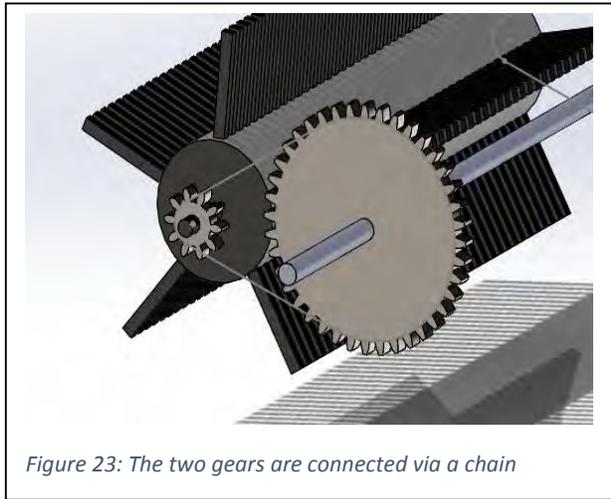
the FRM prototype, a bicycle's front derailleur is used for the larger gear connected to the drive wheel and a one way gear is used for rotating the bristle system. They are connected together using a bicycle chain for the prototype purposes (Figure 23). The drive wheel's larger gear is directly connected to one of the drives wheels by a square, hollow piece of steel. This piece of steel is mounted
