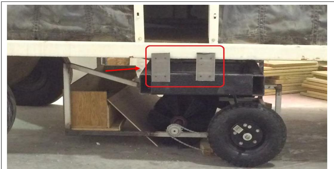
Figure 20: The sheet metal bolted to the flange of the horizontal frame and the flange of the baggage cart
