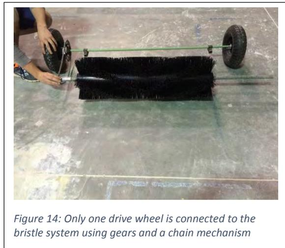
Figure 14: Only one drive wheel is connected to the bristle system using gears and a chain mechanism
