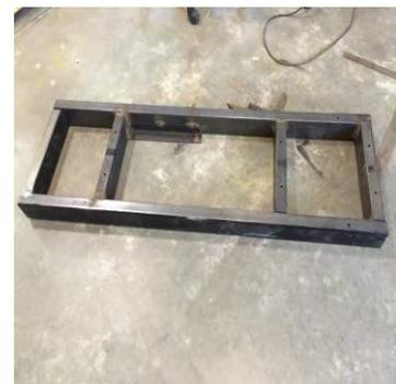
Figure 19: The horizontal metal frame
