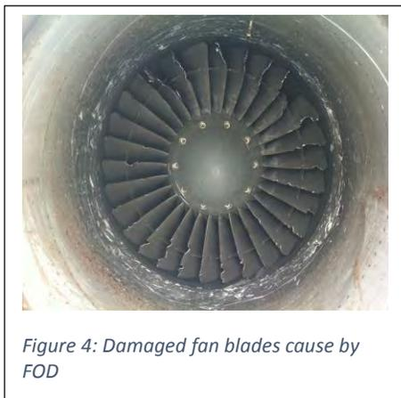
*Figure 4: Damaged fan blades cause by FOD*
