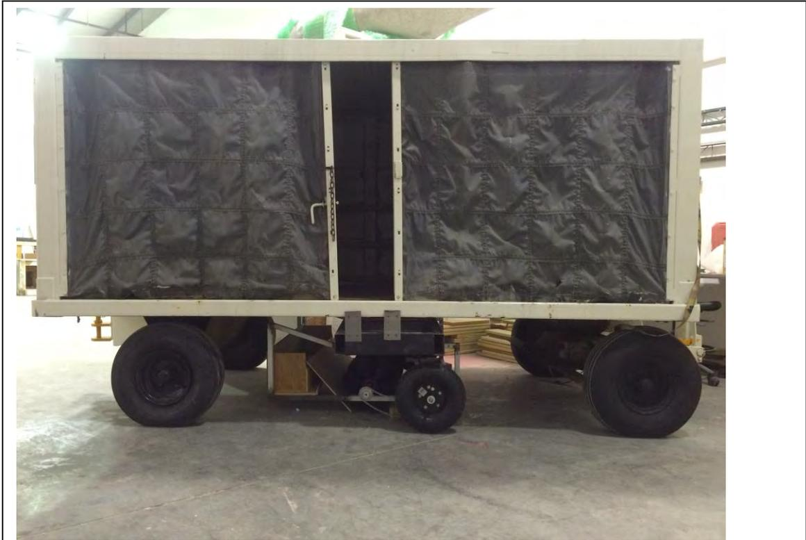
*Figure 11: The final FRM prototype in place under a baggage cart*
