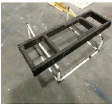
Figure 18: The horizontal frame welded to the framework
