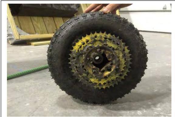
Figure 15: The gear driving drive wheel
