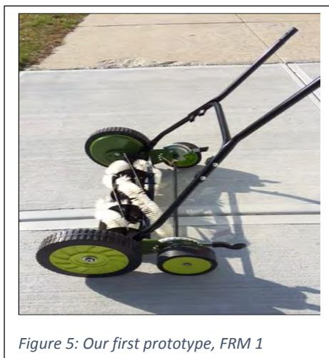
prototypes. Our first scaled prototype, FRM 1, was created with a manual push lawnmower (Figure 5). This was chosen because the rotation of the blades to cut grass is powered by the rotation of the drive wheels, and does not require a motor; instead, a simple interior gear ratio mechanism allow the blades to rotate at a much faster angular velocity than the drive wheels, creating an efficient
