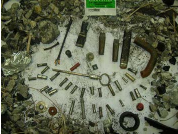
Figure 1: Example of FOD found on runways. [3]
