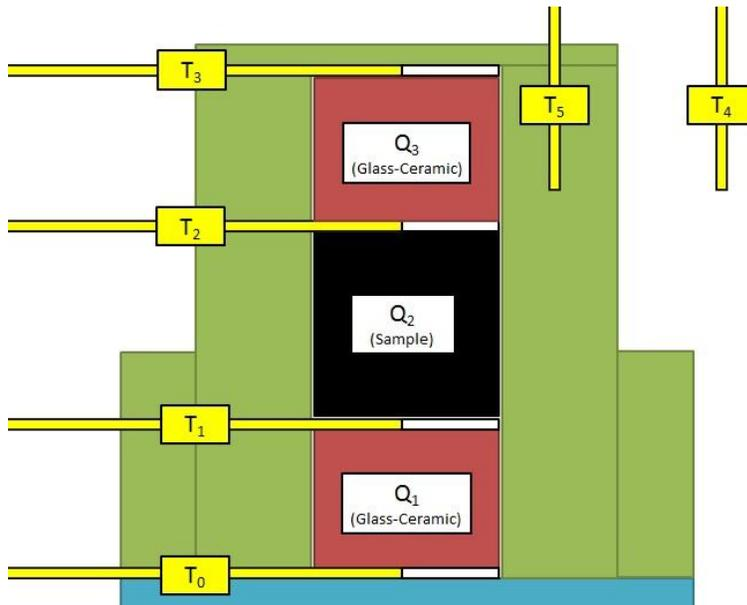
Figure 8: Diagram of the Guarded Longitudinal Calorimeter (GLC) device.
