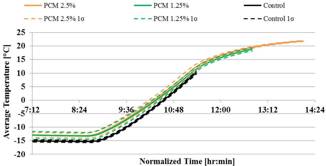
Figure 16: Trial averages at approximate phase change temperature (thawing).
