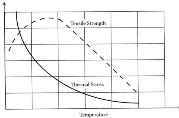
Figure 6: Concept graph of the relationship between tensile strength, thermal stress, and temperature in HMA.<sup>7</sup>
