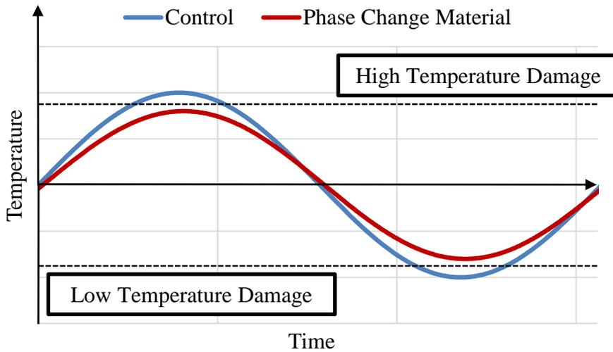
Figure 3: Theoretical illustration of the effect of a PCM on the material temperature profile.
