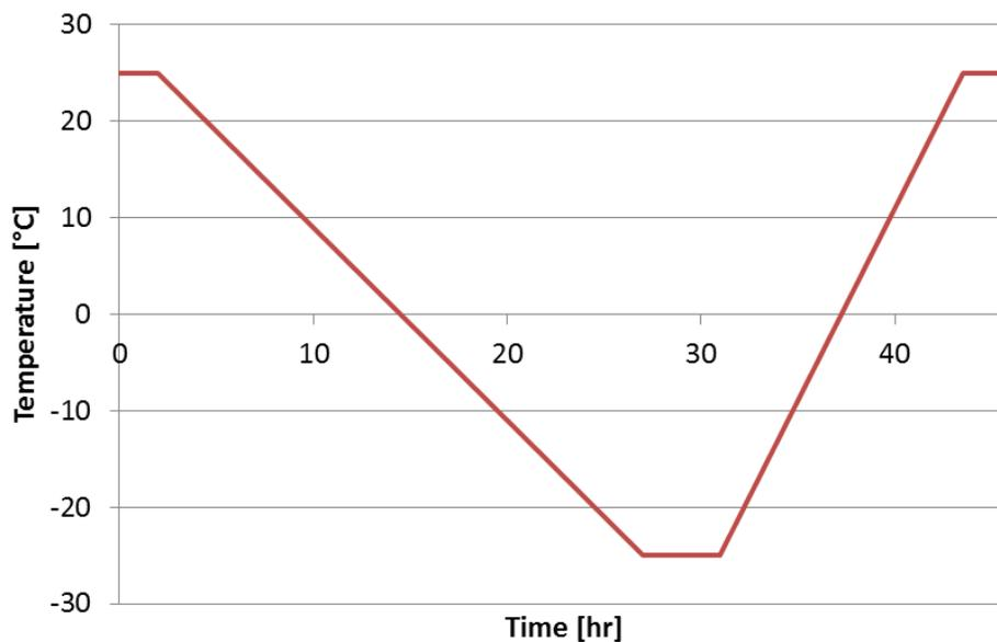
Figure 10: GLC cycle for Phase 3 thermal property testing.
