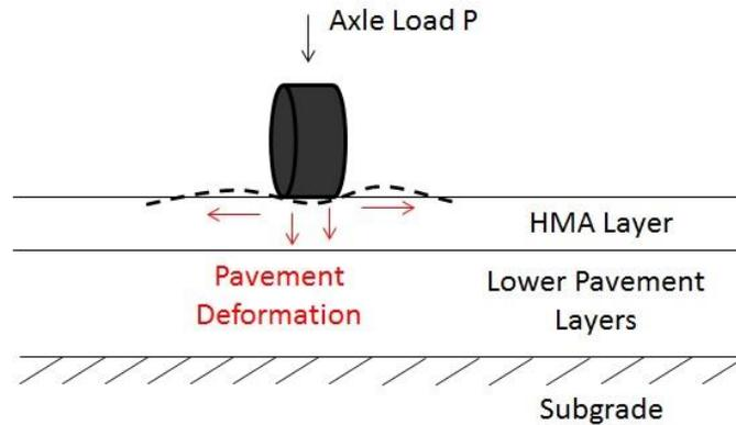
Figure 4: Schematic showing the action of repeated wheel loads over time to create rutting in HMA.
