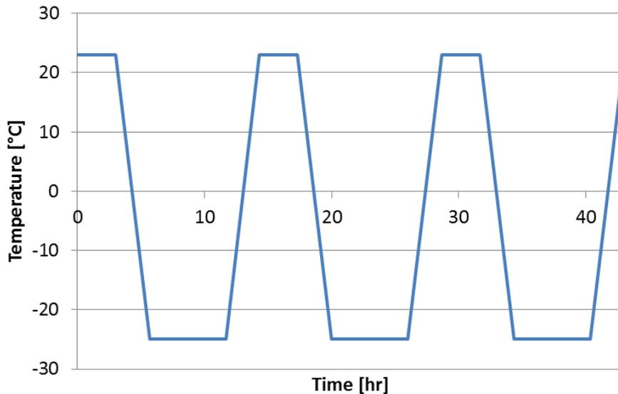
*Figure 9: GLC cycle for Phase 2 thermal property testing.*
