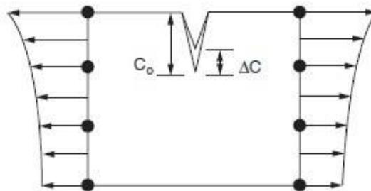
Figure 7: Thermal stress gradient in an HMA layer which causes top-down cracking.<sup>9</sup>
