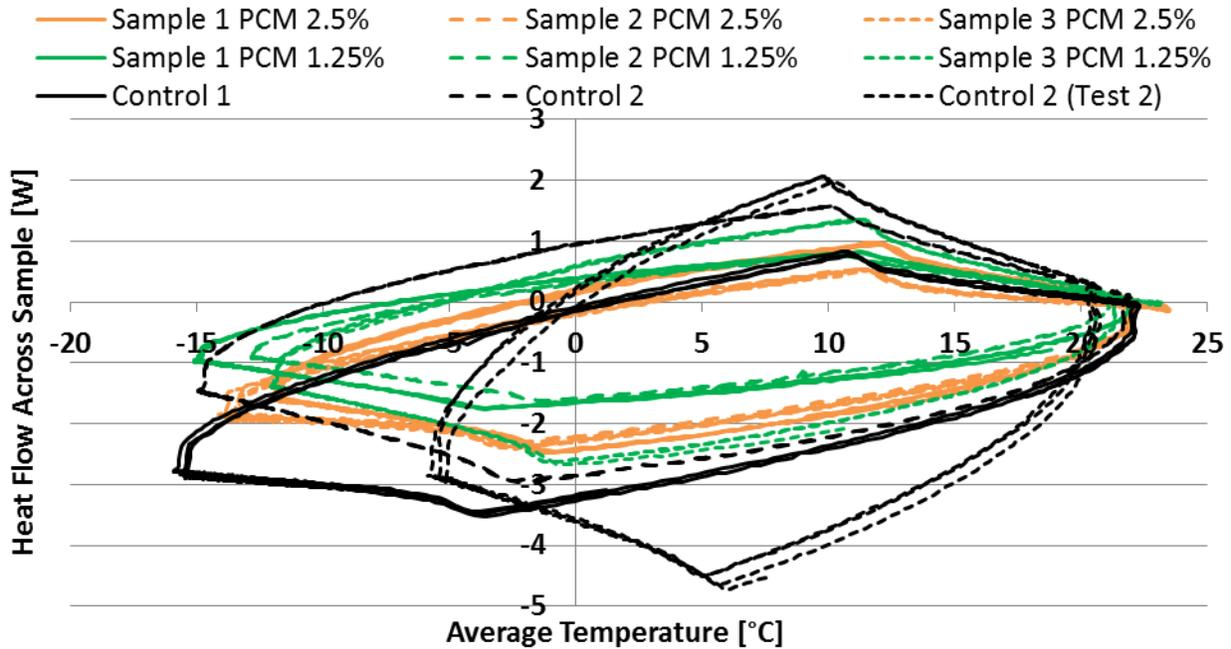
Figure 13: Phase 2 heat flow versus average temperature for samples.
