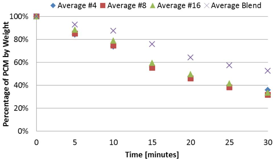
Figure 11: Second PCM-6 evaporation test.
