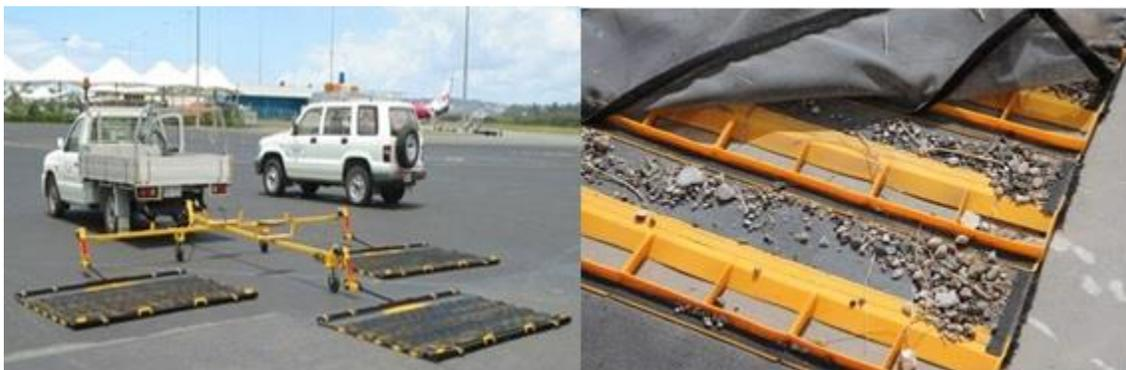
*Figure 1: FOD sweepers commonly used at airports.<sup>4</sup>*
