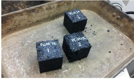
Figure 12: Compacted HMA samples with 1.25% PCM-6.
