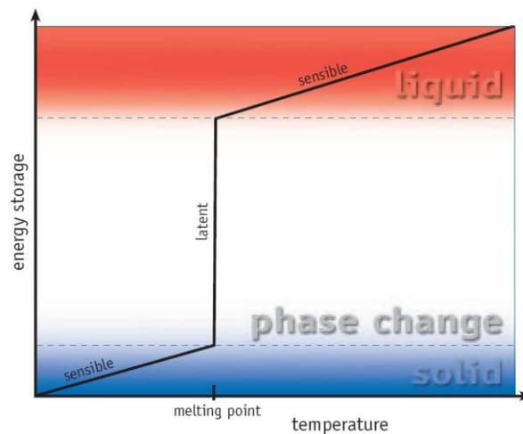
Figure 2: Latent heat versus sensible heat energy storage in a PCM.<sup>6</sup>
