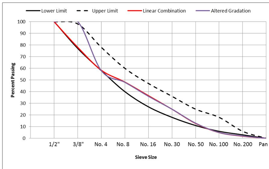
Figure 17: Plot of aggregate gradations for HMA mixes.
