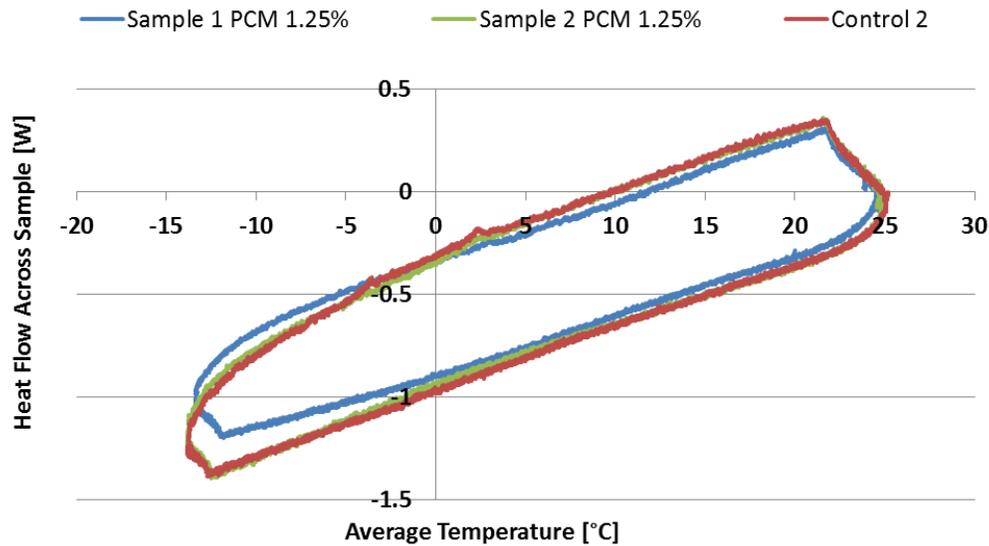
Figure 18: Phase 3 heat flow versus average temperature for samples.
