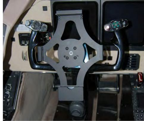
**Figure 6-2. Yoke Mount Fully Installed**
