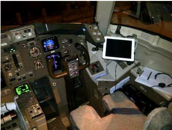
**Figure 6-3. Mounting Solution for Commercial Aircraft**
