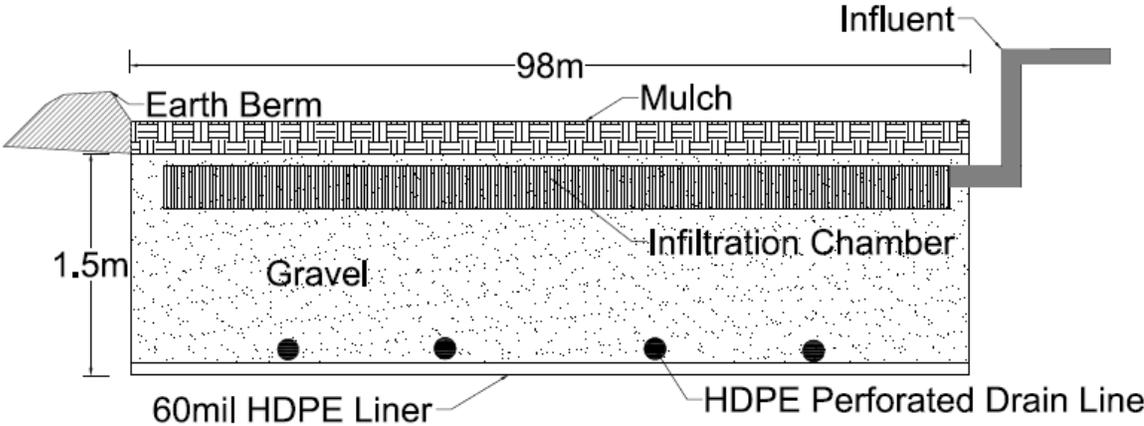
**Figure 8: Cross-sectional view of the length of the aerated gravel bed design**
