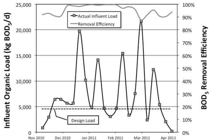
**Figure 2: Influent organic load and BOD removal efficiency for aerated gravel beds at BNIA (Liner)**
