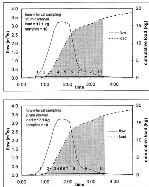
Figure 5: Sample comparison of sampling intervals for time- and flow-interval sampling (R. D. Harmel, 2003)
