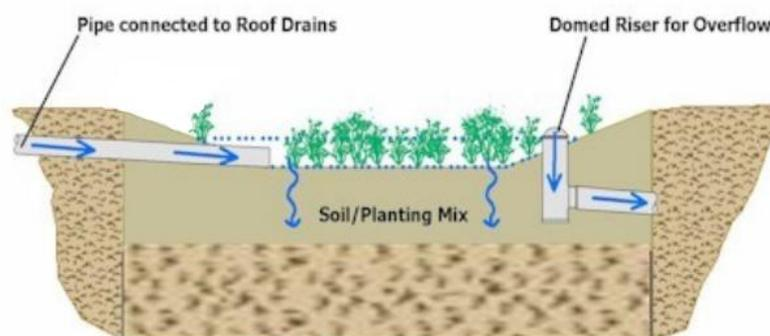
Figure 4: Infiltration basin cross-section (Stormwater PA, 2006)
