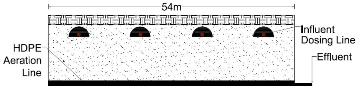
**Figure 9: Cross-sectional view of the width of the aerated gravel bed design**
