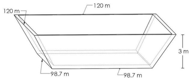
**Figure 10. Side view of retention pond. The top would be ground level and interior surfaces lined with HDPE. Not to**
