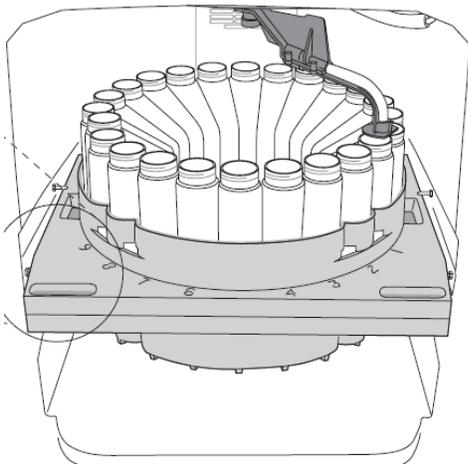
**Figure 7: The bottle configuration within the ISCO 4700 (Teledyne Isco, Inc., 2008)**
