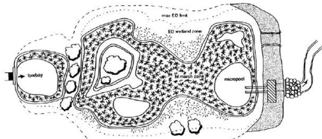
Figure 3: Schematic of engineered wetland (Schueler, 1992)
