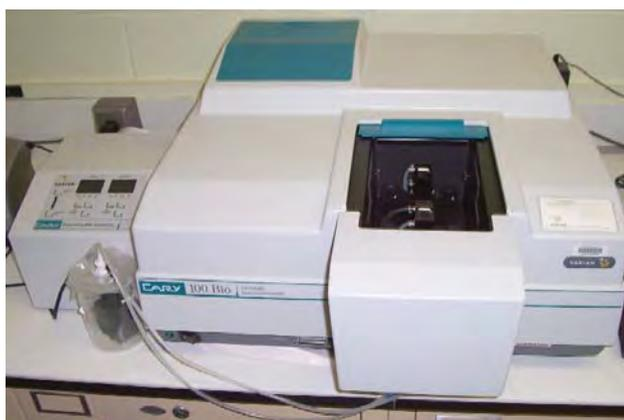
**Figure 4. UV-Vis Spectrophotometer**
