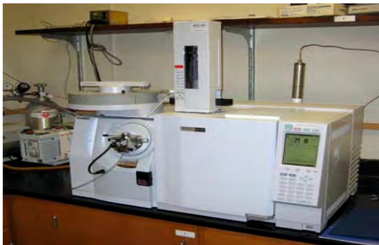
**Figure 6. Gas Chromatograph-Mass Spectrometer**
