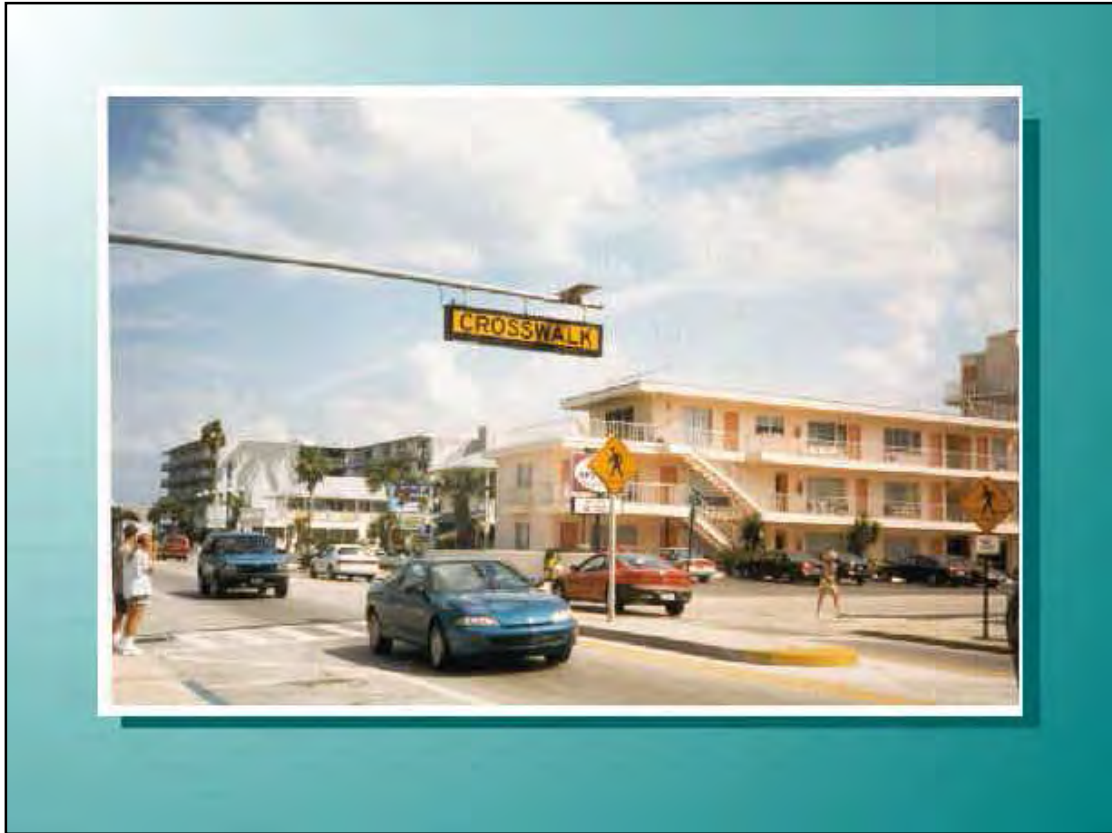
Figure 14: Illuminated overhead crosswalk sign (Nitzburg and Knoblauch, 2001)
