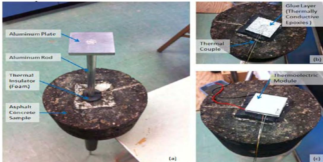
Figure 2.1: Experimental set up of thermoelectric energy harvester (1)
