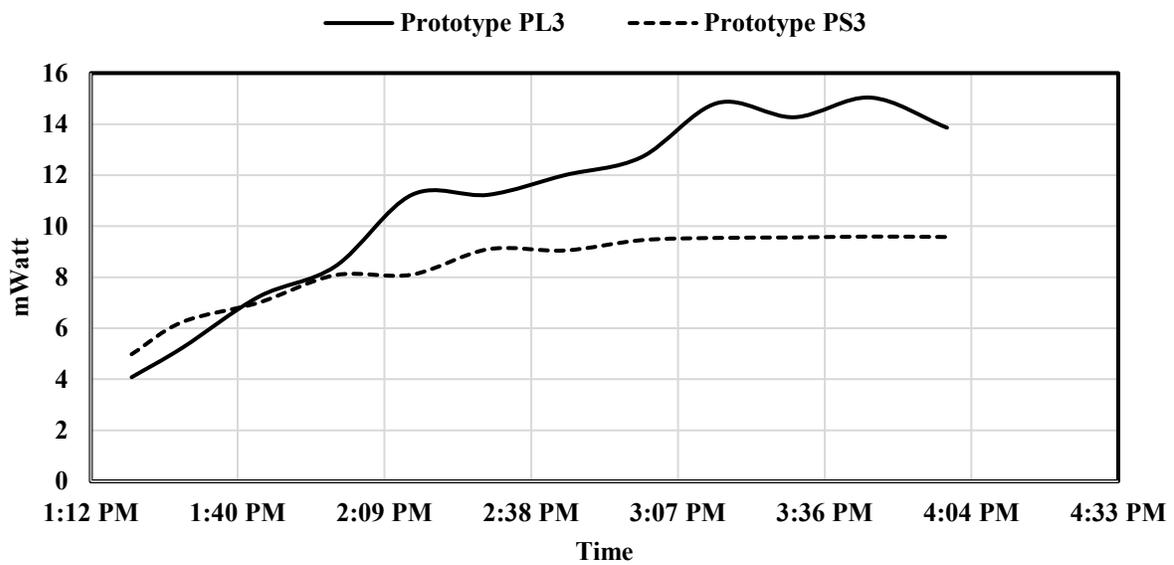
Figure 5.18: Field results during day time showing output power of Prototype PL<sub>3</sub> and PS<sub>3</sub>
