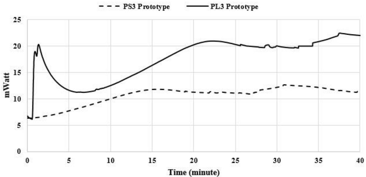
Figure 5.10: Lab result of output power with time for PL<sub>3</sub> and PS<sub>3</sub> Prototype
