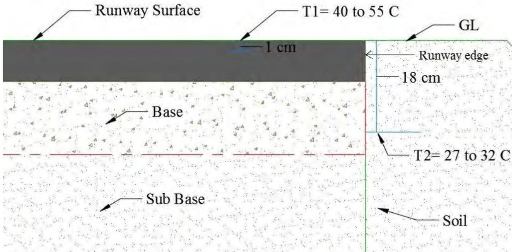
Figure 3.2 Pavement and soil temperature
