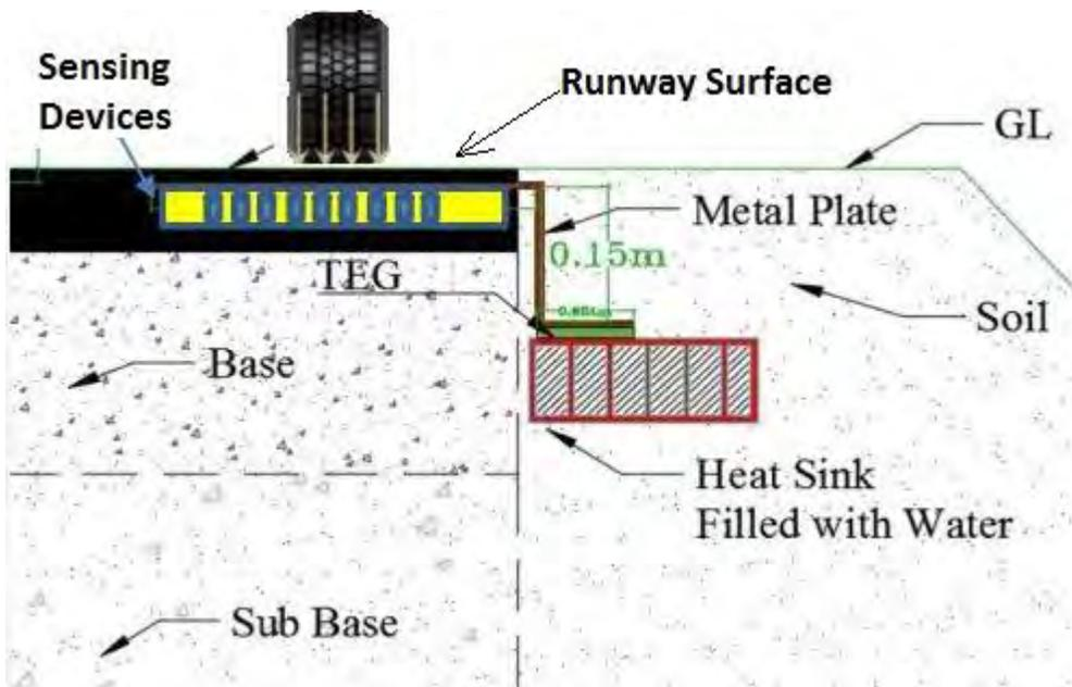
Figure 3.3: Energy harvesting prototype at runway edge
