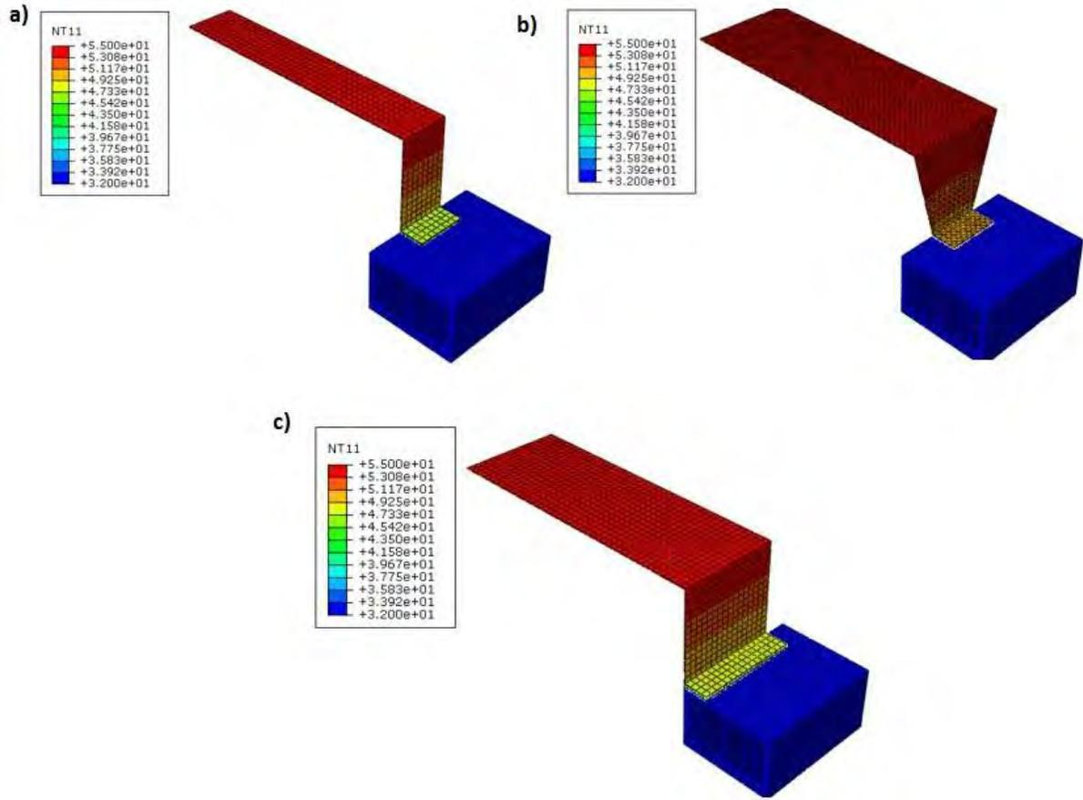
Figure 5.2: Finite element analysis on a) Ps<sub>1</sub> b) Ps<sub>2</sub> and c) Ps<sub>3</sub> Prototype
