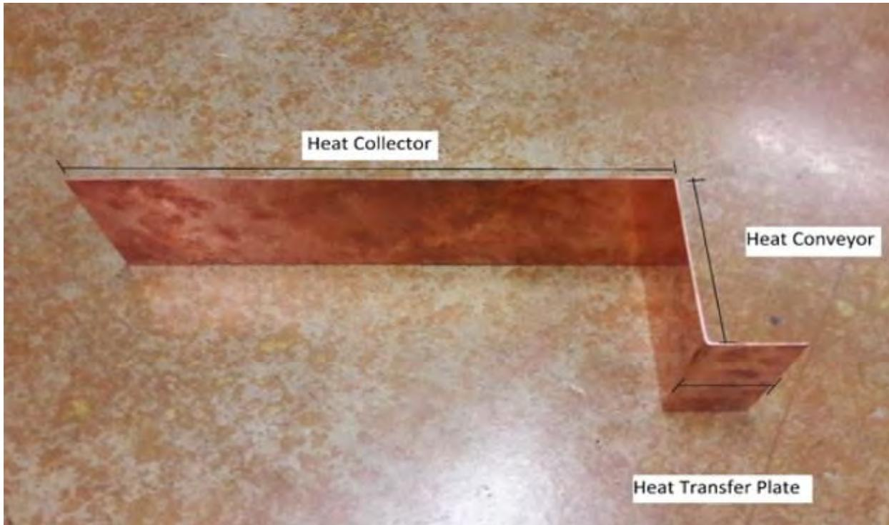
Figure 3.5: Heat conducting metal plate
