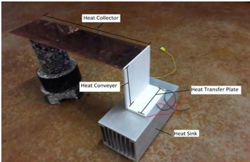
Figure 3.4: Heat energy harvester
