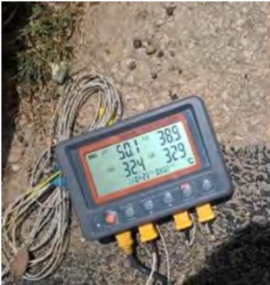
Pavement Surface Temperature,  $T_1 = 50.1^{\circ}\text{C}$
