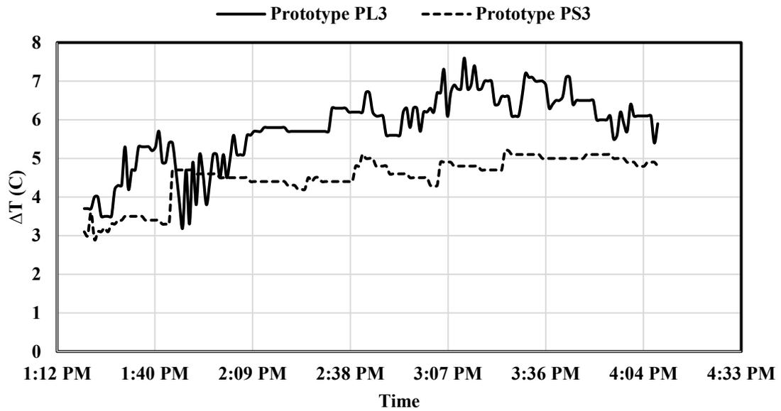
b) Temperature gradient for Prototype PS<sub>3</sub> and PL<sub>3</sub>
