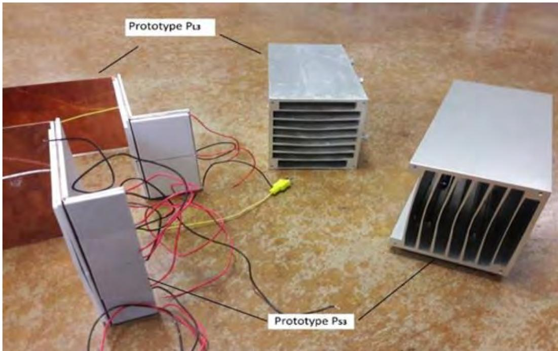
Figure 5.3: Prototype  $P_{L3}$  and Prototype  $P_{S3}$  fabrication for lab experiment
