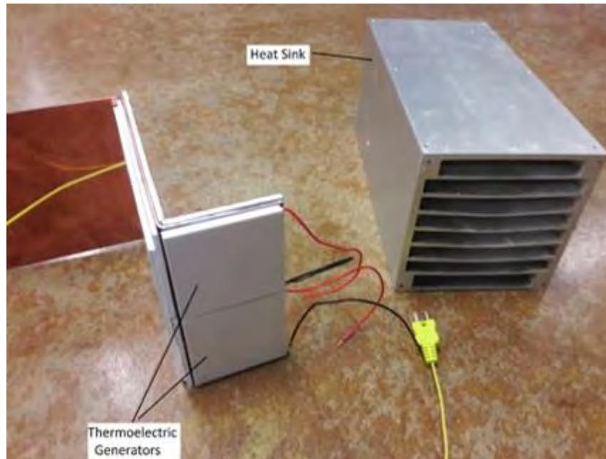
Figure 3.6: TEGs attached with heat transfer plate and Heat Sink
