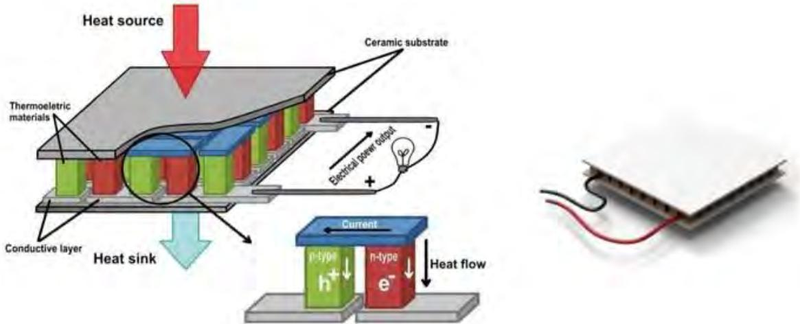
Figure 3.7 Schematic diagram of the internal components of TEG (10)
