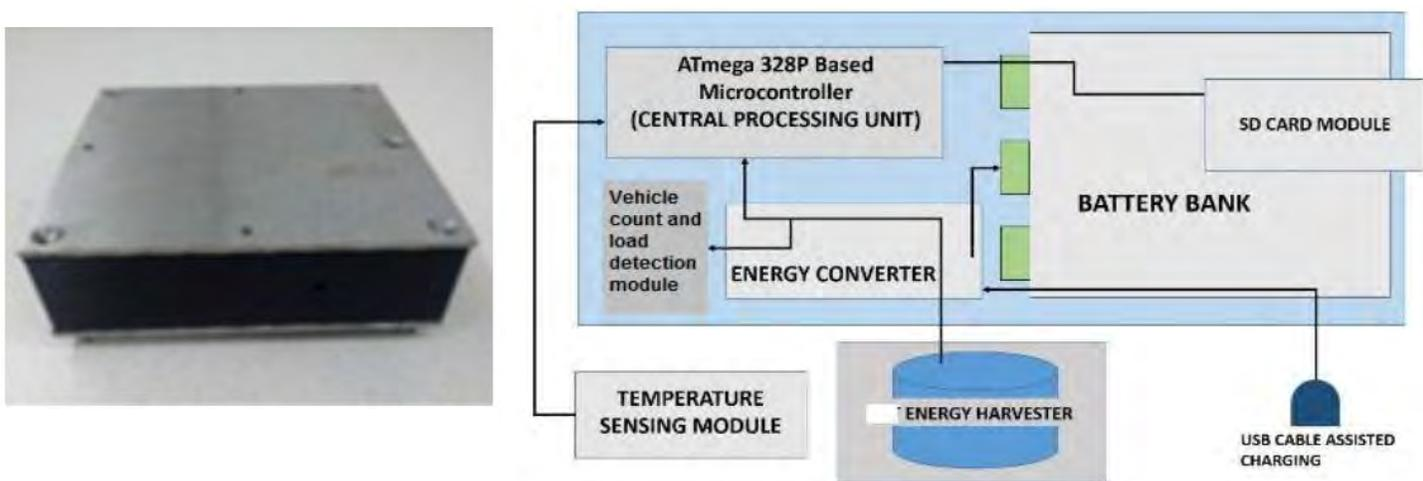
**Figure 5.19.** a) Sensing enclosure to seal sensors and electronic components b) Block diagram of micro-power sensing and data logging module
