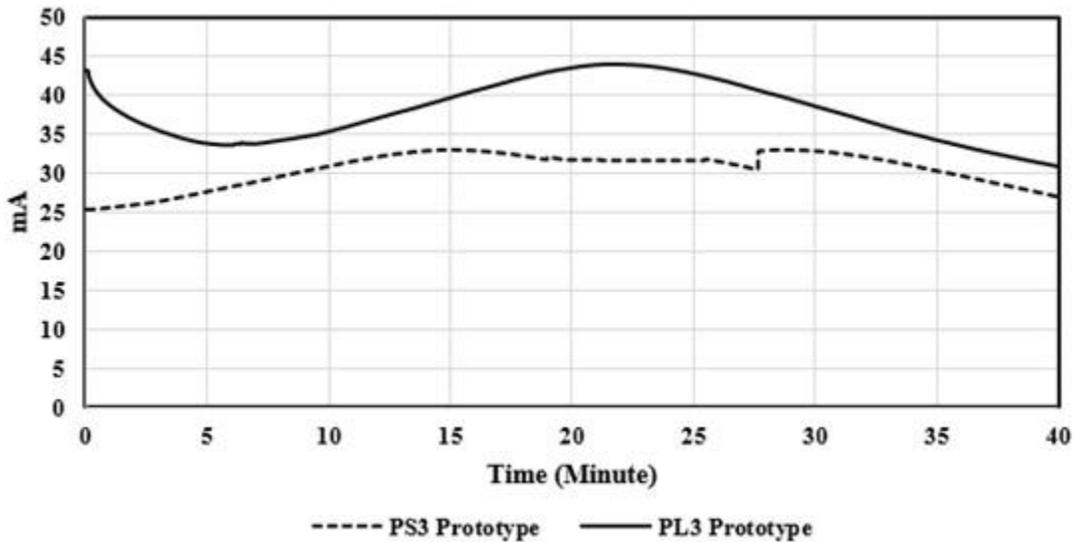
Figure 5.9: Lab result of output current with time for PS<sub>3</sub> and PL<sub>3</sub> Prototype
