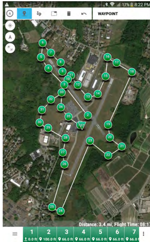
Figure 4: Perimeter flight path at Newport State Airport
